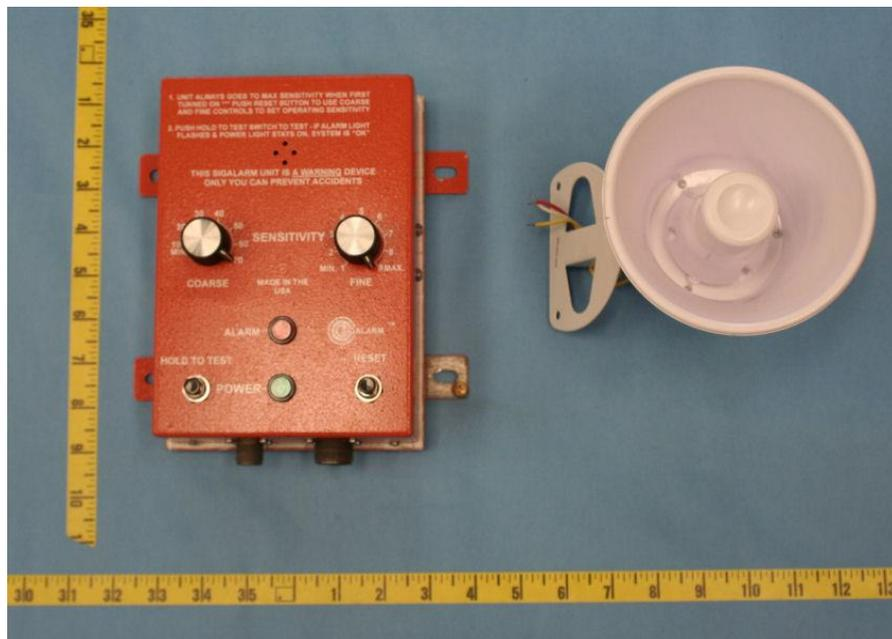
Figure 4. Sigalarm controller and alarm horn.
