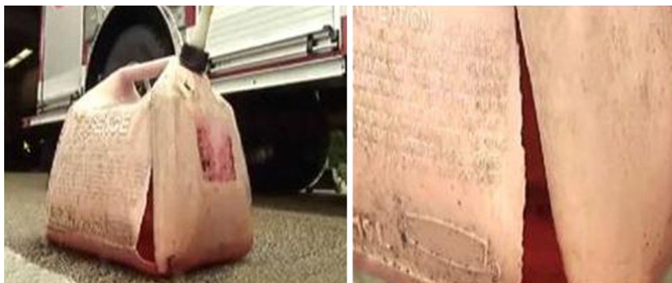
Fig. 1 A PPGC shown in news footage following a fire incident. Damage demonstrates fractures consistent with explosion and rupture having occurred
