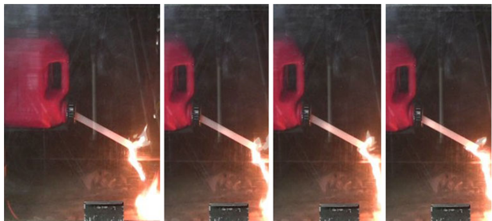
Fig. 8 Stills from a high-speed video of a 2-gallon (7.85-L) can test showing the flame traveling up the translucent plastic spout and confirming a flame speed of approximately 0.4 m/s
