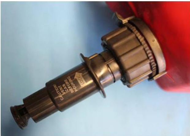
Fig. 12 Child-resistant, automatically closing nozzle jammed in open position
