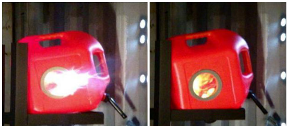
Fig. 6 Gasoline cans tested w/o flame arresters (6-19-08: tests 7 and 8)
