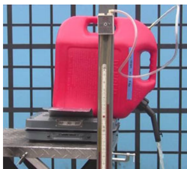
Fig. 4 Gas can monitored by monometer (left) during pouring from a 5-gallon (18.93-L) PPGC. A typical plot of time vs. vacuum pressure measured is plotted at the right side
