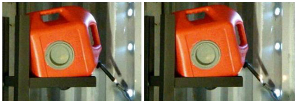
Fig. 11 Gasoline cans tested with flame arresters exhibited no explosion in spite of flame travel up nozzle
