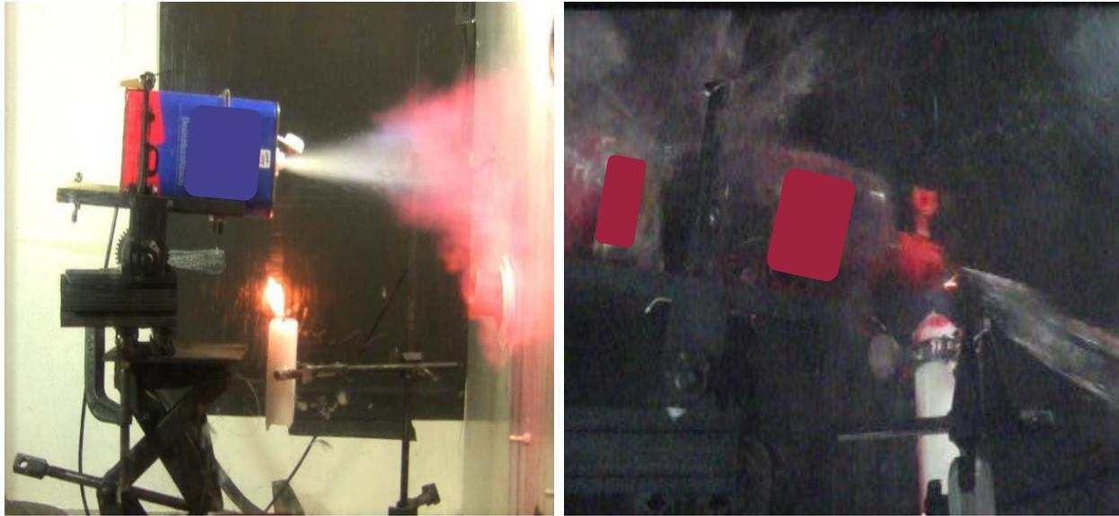
Figure 10. (a) Combustion testing of alcohol container and (b) a gelled alcohol container which ruptured.
