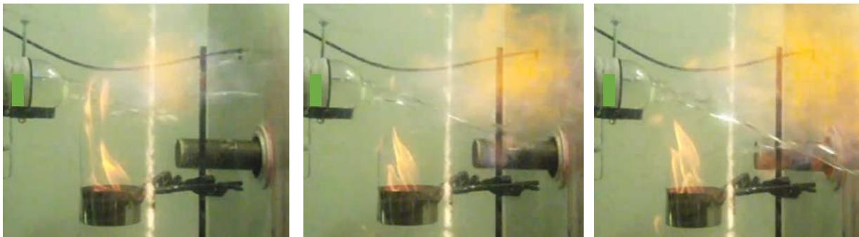
Figure 1. Vapor space inside a gelled alcohol container ignited by an external flame producing a dangerous jetting action. Testing performed at BEAR.
