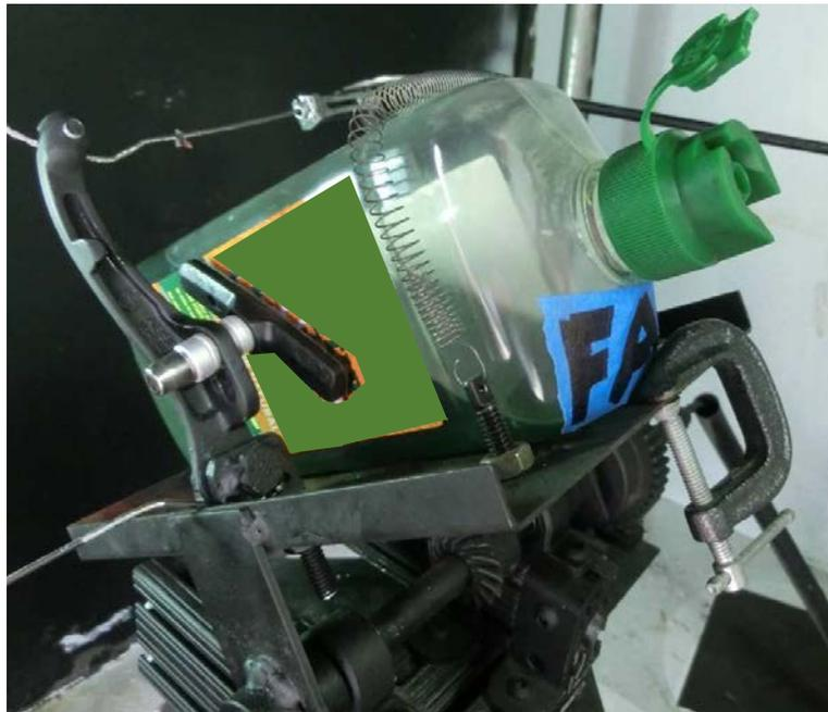
Figure 5. Test Setup – Tipping and Squeezing platform assembly with a Manufacturer A Container mounted for testing.
