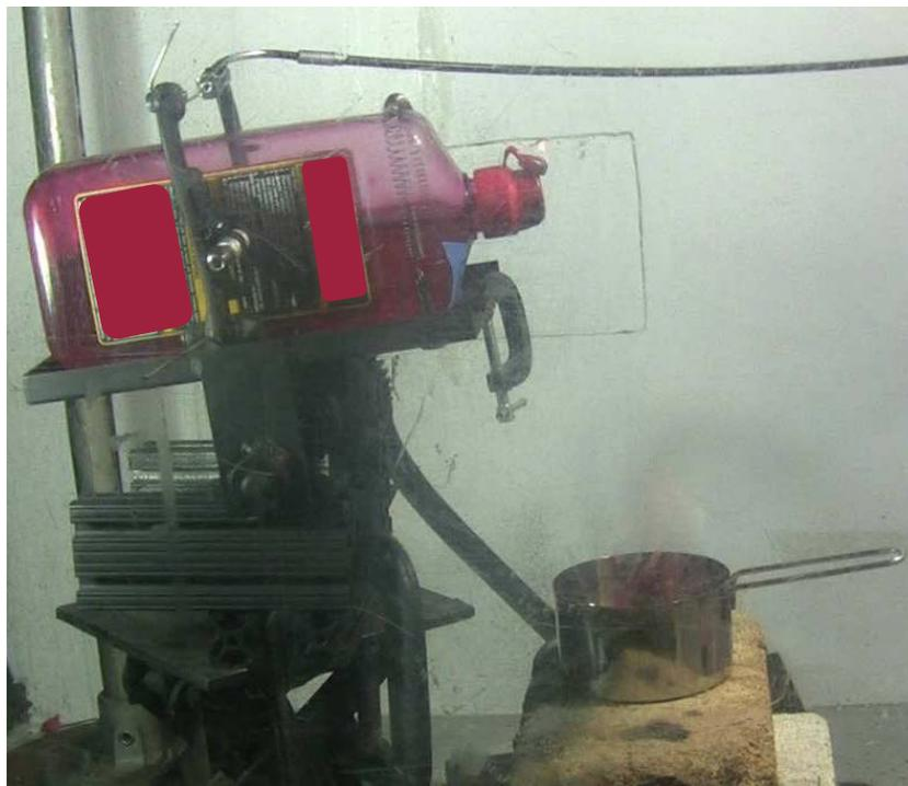
Figure 8. Manufacturer B container with a flame arrestor during testing. Opening exposed, not covered by alcohol gel.
