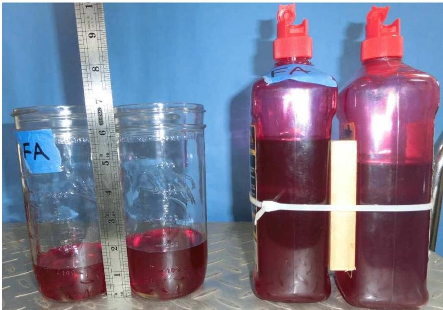
Figure 4. Manufacturer B Containers showing a difference in pour rate with and without a flame arrestor in the cap.
